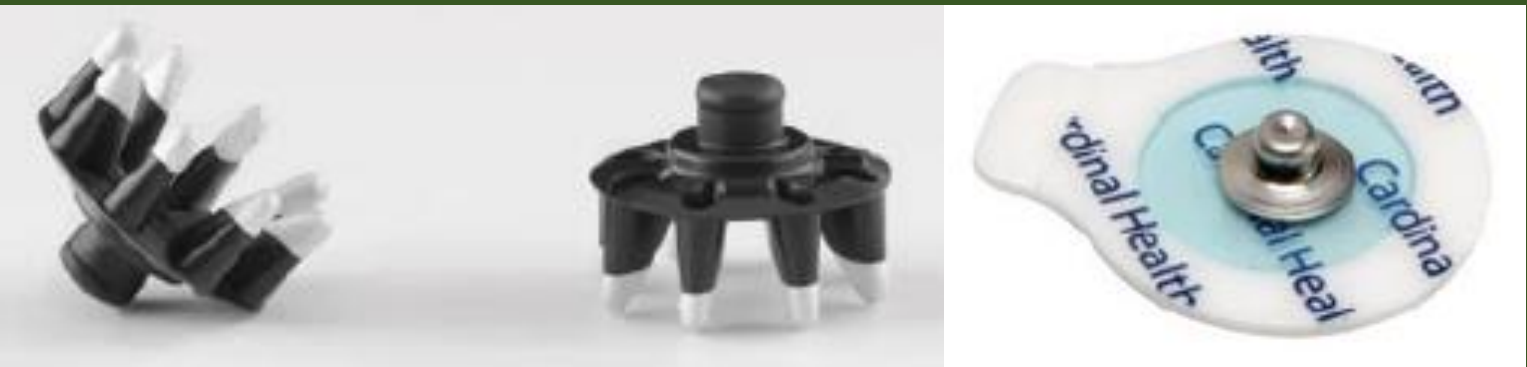
Figure 2. A: Dry electrodes. B: Conventional gel-based electrodes.
