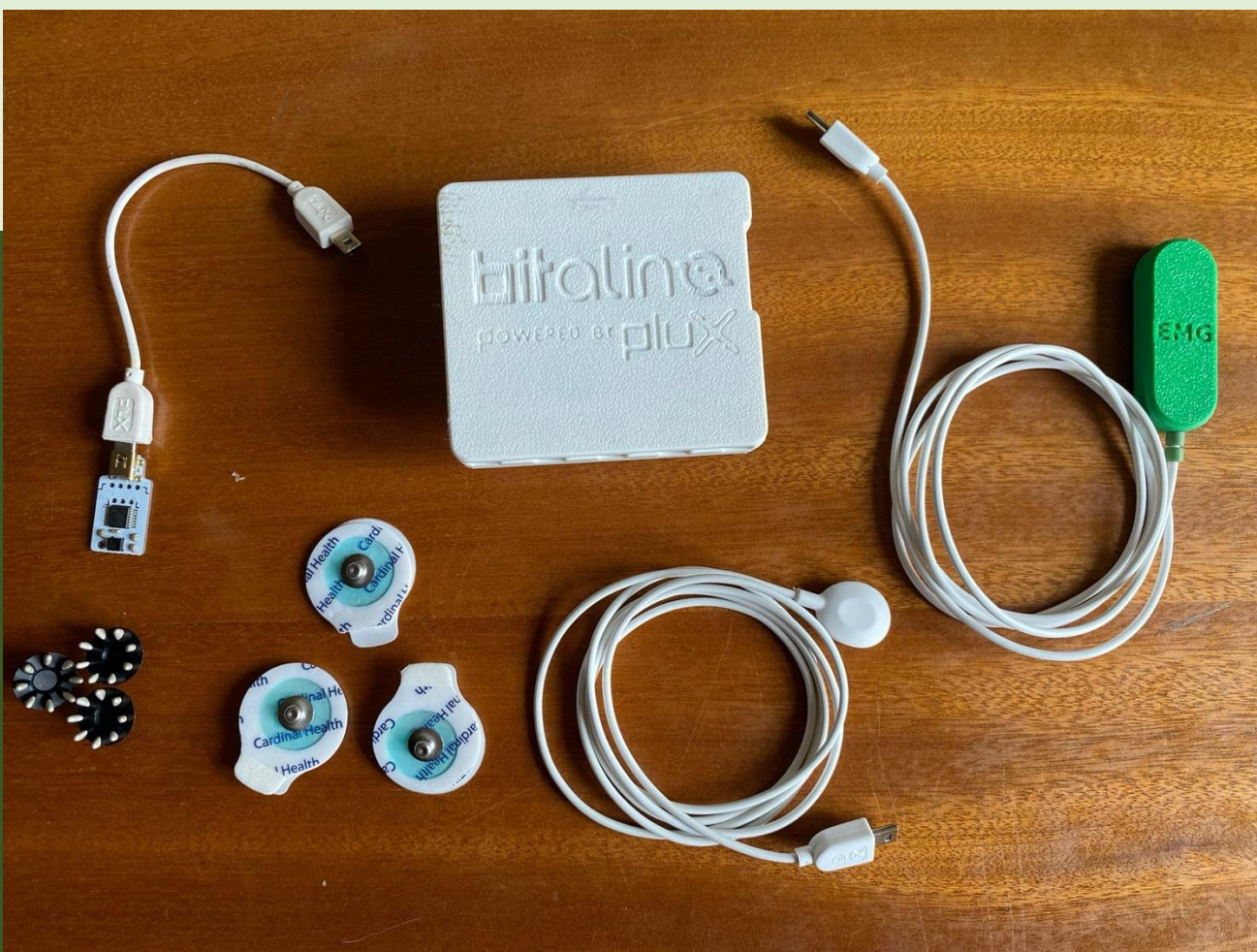
Figure 1. sEMG setup - BITalino® EMG, Portugal.
